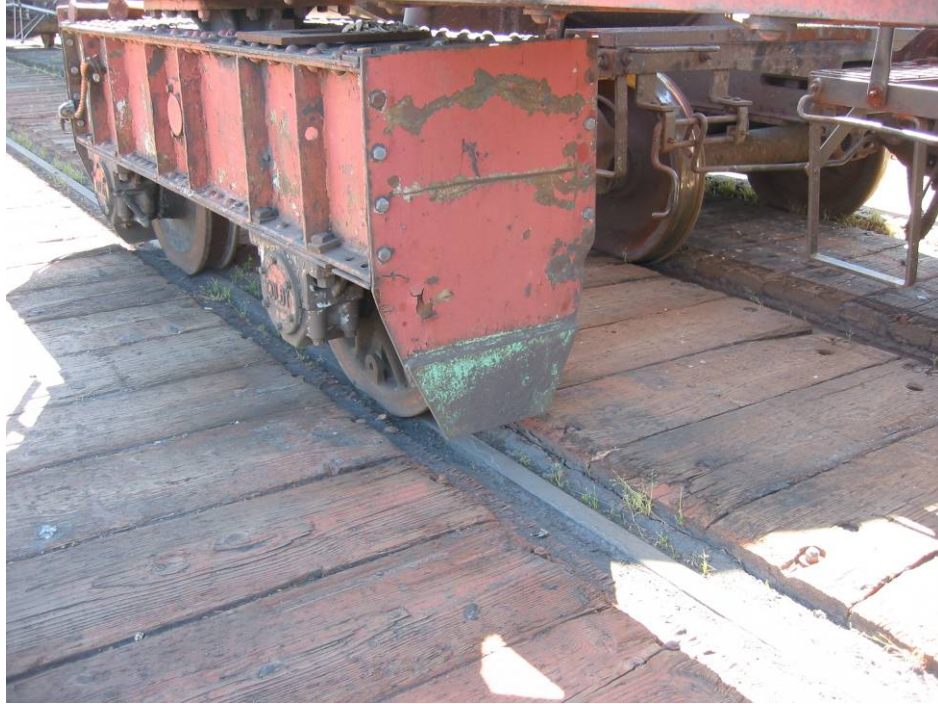
One of the our self-propelled “trucks” that carry the whirly crane on a pair of steel rails
