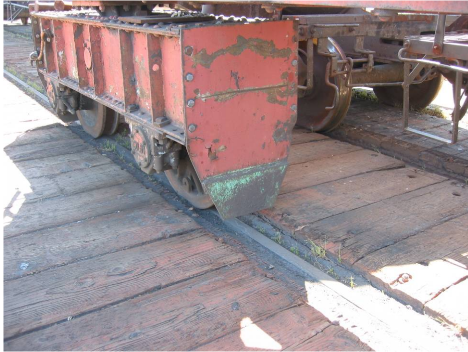
One of our self-propelled "trucks" that carry the whirly crane on a pair of steel rails
